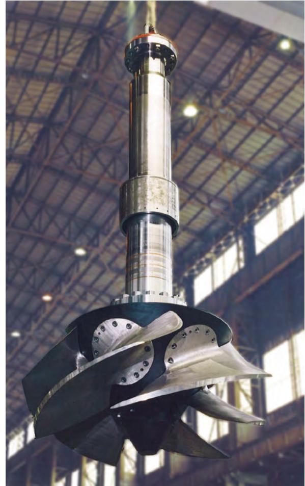
Impeller of main pump installed in the drainage pump station (Impeller diameter is 3,757 mm)
