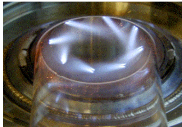
Special burner of combustion abatement system
