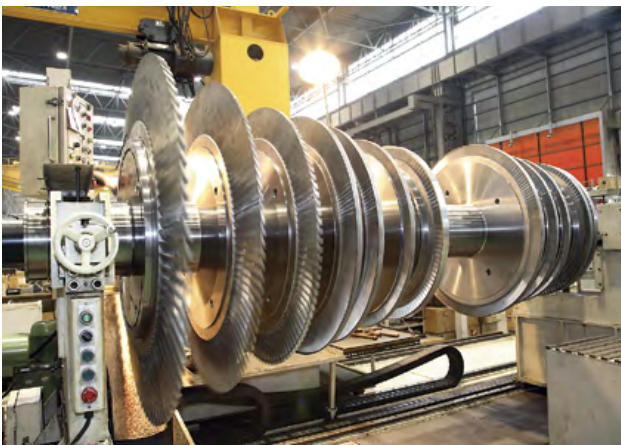
Assembly of multistage turbine rotor blades
