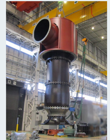
A water intake pump for a power station
