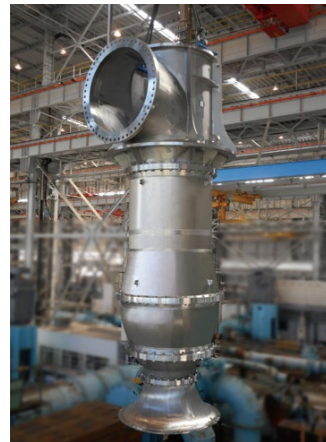
Vertical mixed flow duplex stainless-steel can pump with adjustable vane
