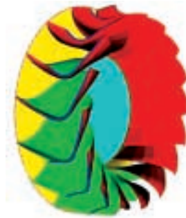
図9 逆解法設計ランナの3次元形状 Fig. 9 3-D geometry of inverse design runner
