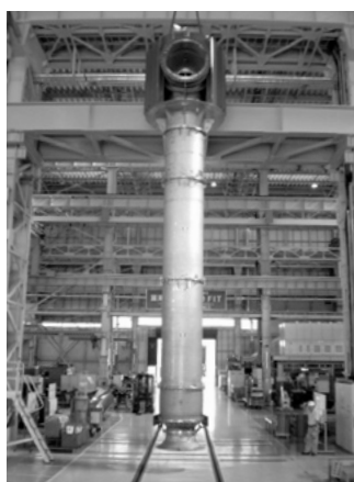
写真6 1100 mm 立軸斜流ポンプ Photo 6 Vertical mixed flow volute pump 1100 mm bore
