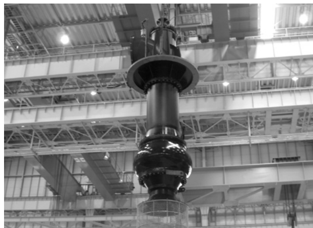
写真7 1000 mm 立軸斜流ポンプ Photo 7 Vertical mixed flow volute pump 1000 mm bore
