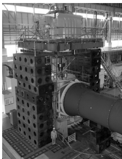
写真3 3000 mm立軸斜流ポンプ Photo 3 Vertical mixed flow volute pump 3000 mm bore
