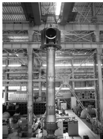
写真8 1000 mm 立軸斜流ポンプ Photo 8 Vertical mixed flow volute pump 1000 mm bore
