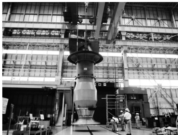
写真14 1800 mm 立軸斜流製缶ポンプ Photo 14 1800 mm vertical mixed flow can pump
