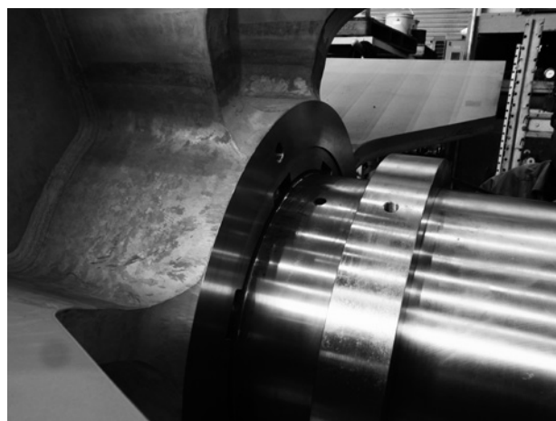
写真37 加熱炉排ガス用高温送風機の回転体 Photo 37 Rotating body of hot air fan for gas discharged from heating furnace
