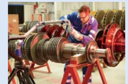
Steam turbine undergoing repairs
